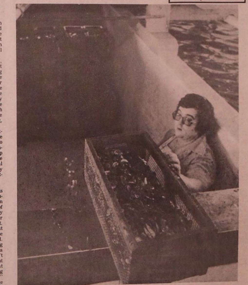
From the depths of a 3,000 gallon purification plant, Paul Knox grabs a box of clams and stacks it with others. When the tide reaches its peak for the day, the tank will be flooded with purified sea water.
